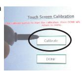
Press and briefly hold the stylus on the center of the target, then release. Repeat as the target moves around the screen.
