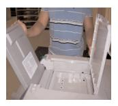
Remove the clean-out tray by pushing in on the flat round tabs at the sides and rolling it forward towards the screen.
